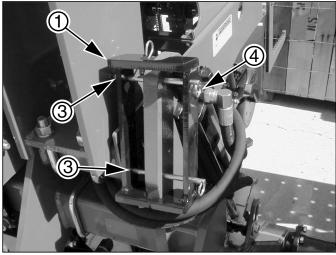
Figure 15: 2011-Lift Cylinder Lock Storage
