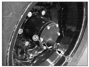
Figure 17 Lock-Out Hub Engaged
