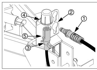
Figure 27 Hose and Connector Storage
