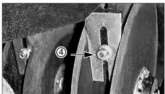
Figure 38 Disc Scraper Adjustment
