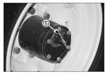
Figure 18 Lock-Out Hub Disengaged
