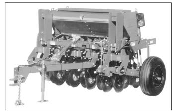
Figure 2 606NT No-Till Drill
