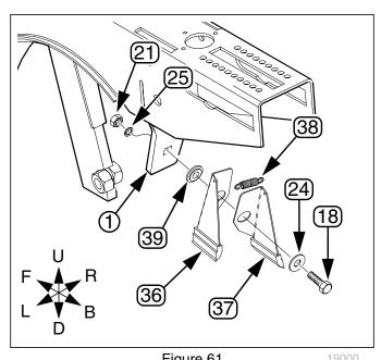
Figure 61 Carbide Disc Scraper Installation
