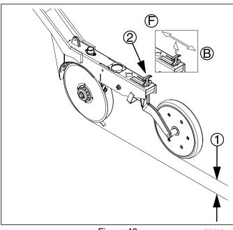
Figure 42 Adjusting Opener Depth
