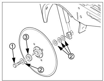
Figure 37 Adjusting Disc Spacers
