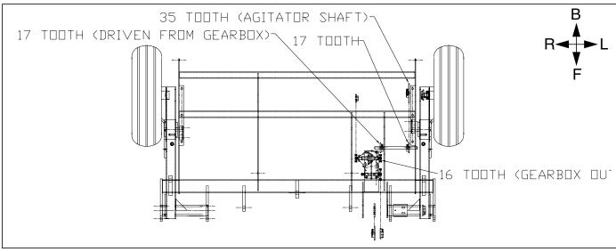
Figure 55 605NT and 606NT Main Seed Box Agitator (Option)
