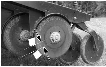
Figure 36 Checking Disc Contact
