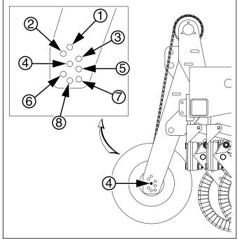
Figure 10 Height Adjustment, 3P605NT or 3P606NT
