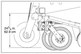
Figure 9 Initial Field Height, 3P605NT or 3P606NT
