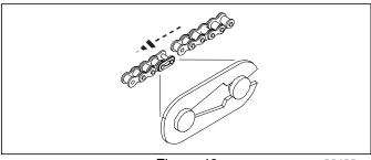
Figure 49 Chain Clip Orientation
