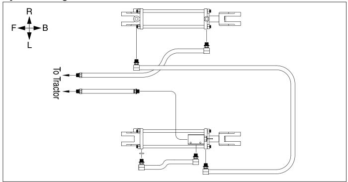
Figure 50 605NT and 606NT Hydraulic Diagram
