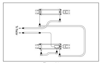
Figure 21 605NT or 606NT Lift Hydraulics
