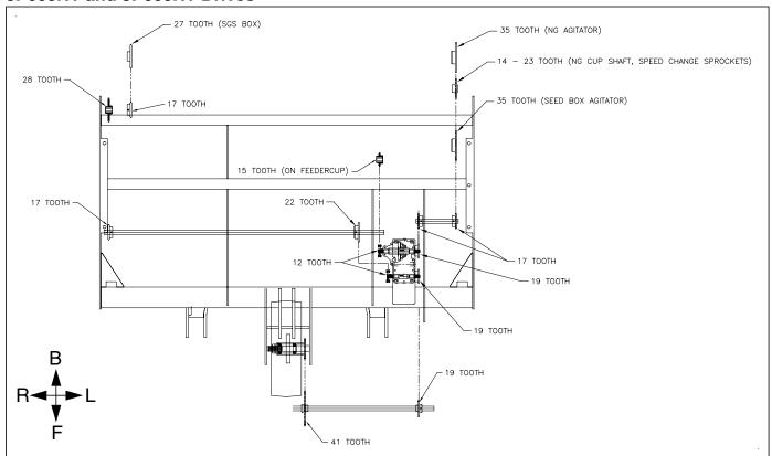
Figure 51 3P605NT and 3P606NT Maximum Configuration
