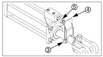
Figure 12 Cylinder Depth Stop
