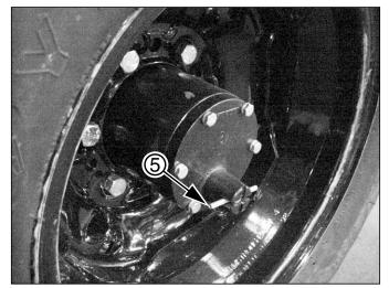
Figure 20 Lock-Out Hub Engaged
