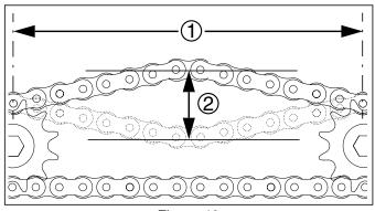
Figure 48 Measuring Chain Slack
